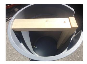
Cut off the handle and rim of the cans on the side where they would be attached to the sheet of ply to make for a flat surface. The bottoms of the two cans are attached together with a bolt to prevent them from moving independently.
