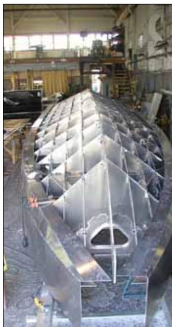
Above: The RCM-SAR 37 Sooke vessel is being built at Kamma and Blake Industries in Port Alberni.
